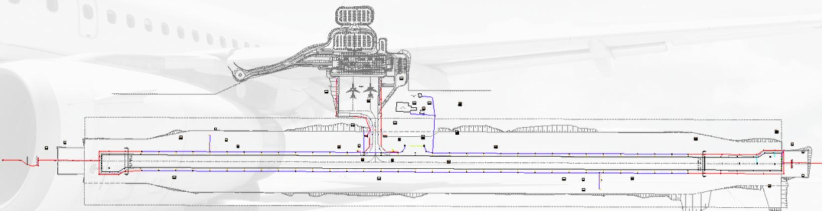
Kumasi International Airport's existing runway was extended on the southern and northern sides, to accommodate the critical design aircraft (Boeing B737-800W (with winglets)). The runway was designed as a code 4D precision approach runway, as per ICAO annexure 14 specifications.
